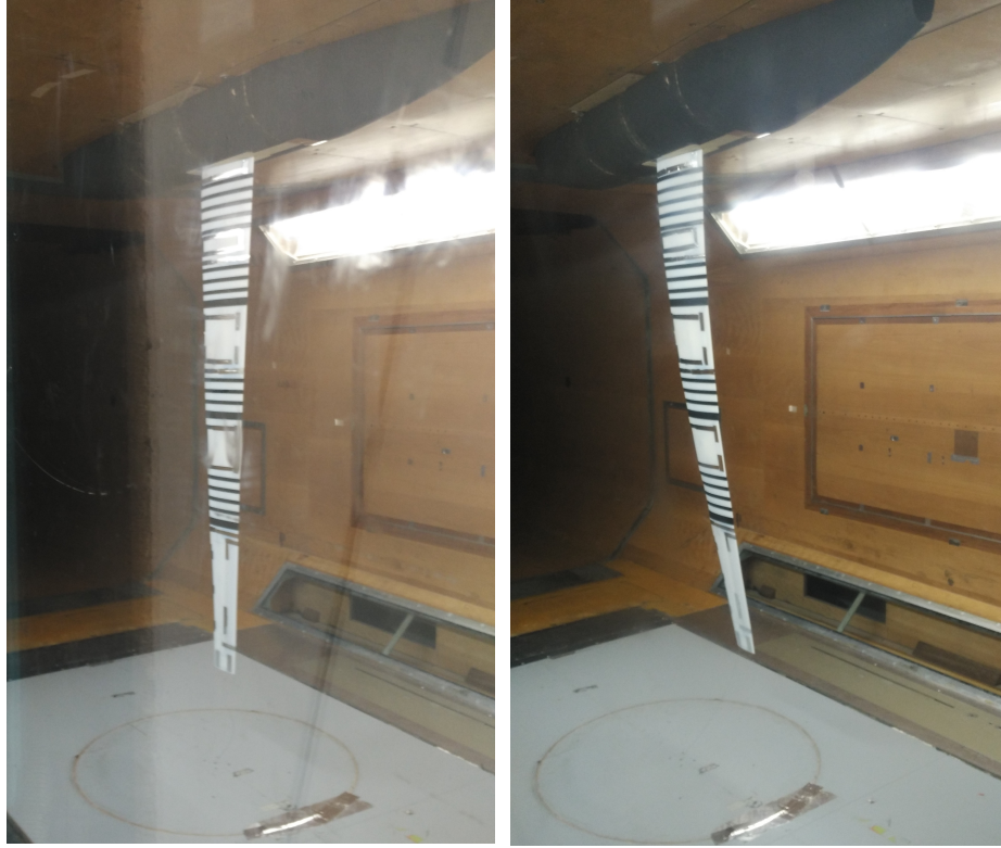
Figure 6.33: The xb-2 wing inside the wind tunnel facility (left: wind speed 0 m/s, right: wind speed 40 m/s).
