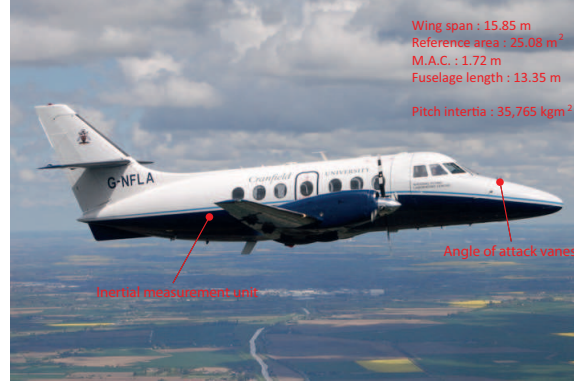
Figure 3.2: Cranfield's Jetstream 31 G-NFLA and reference data.
