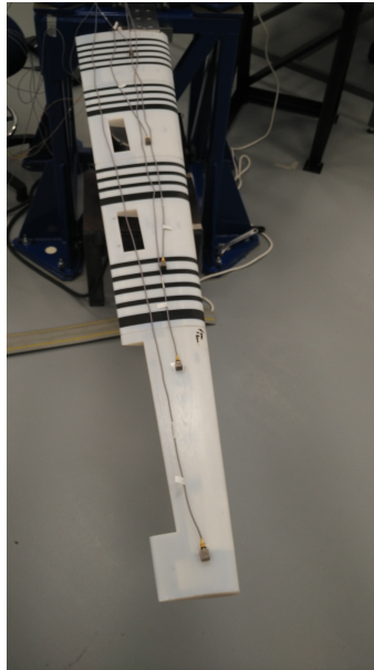
Figure 6.26: Spar and skin GVT setup.
