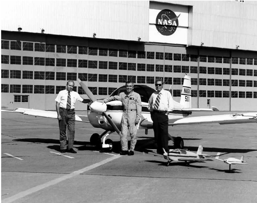
Figure 2.2: Example of different test model used for spin testing. Left to right: full-scale aircraft, radio-controlled model, and spin tunnel model (Reproduced from Reference [10]).
