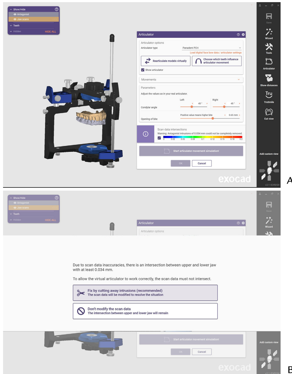
Figure 5. A, Representative articulated specimen mounted on virtual semiadjustable articulator (Panadent Articulator. B, CAD program detecting occlusal collisions among articulated specimens in which two options available: making no changes or trimming the casts.
