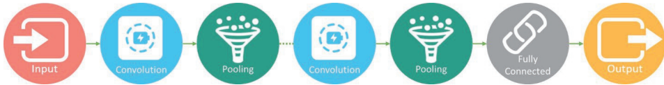
Figure 2.5 Convolution Neural Network (CNN) is a class of Deep Learning (DL) neural networks that is widely used for image classification. A CNN includes an input layer (image data), multiple hidden layers (convolution to extract features, pooling for subsampling features, and fully connected layer to classify images), and an output layer.
