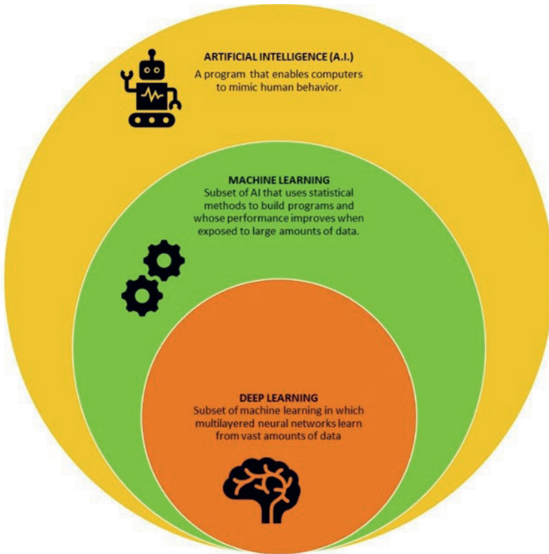
Figure 2.1 The relationship between AI, ML and Deep Learning (DL). ML is a subset of AI and DL is a subset of ML. ML is a sub-discipline of AI that uses training examples of how to perform a specific task without explicit instructions to identify associations for a given outcome measure. DL is a subfield of ML that mimics neural networks to learn.
