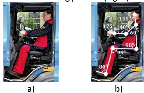
Fig. 2 View of the driver's seat to assess ergonomic factors: a) the location of the driver in the cabin of PB; b) the location of the driver in the cabin of PB with the applied body structure
