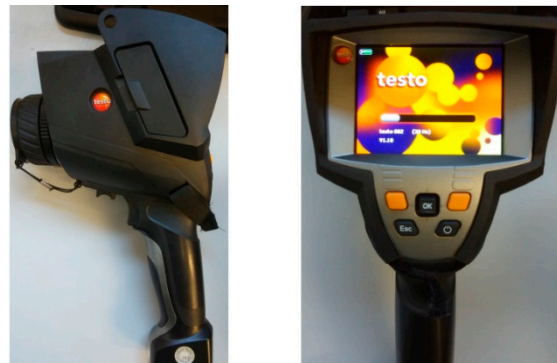
Figure 2. IR camera Testo 882 to measure surface temperature variation used during fatigue tests.
