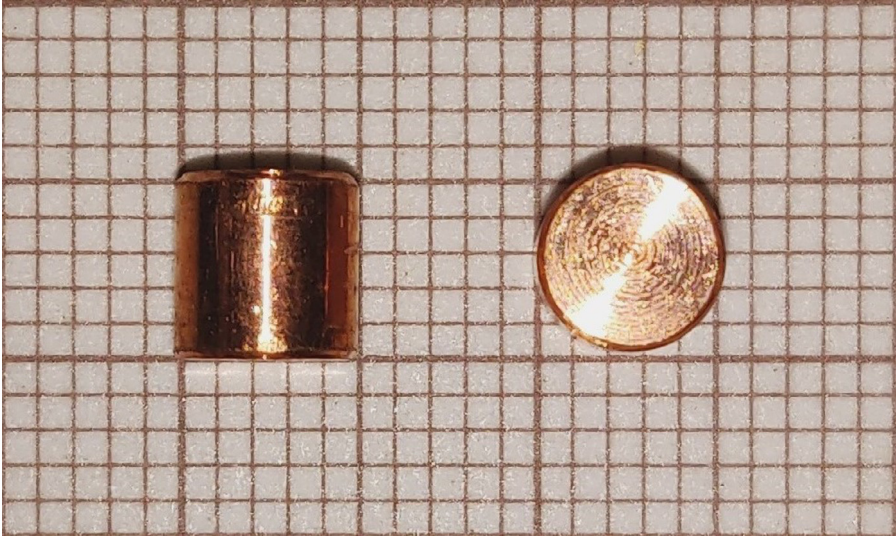
Fig. 3. Pure Cu 5 × 5 mm cylindrical specimens over millimeter paper on the background.
