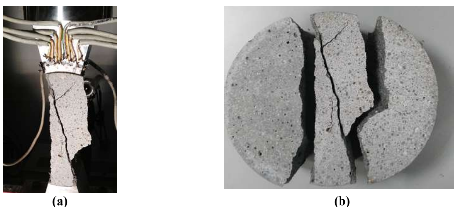
Figure 9 Failed disk sample D_III1
