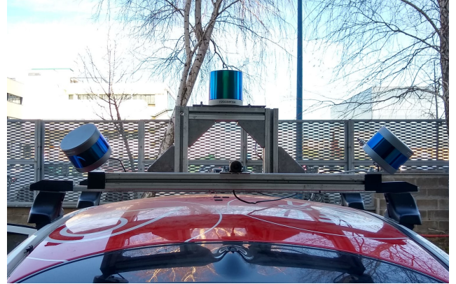
Fig. 6. Autonomous vehicle platform used to perform real experiments with LiDAR sensors attached.
