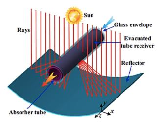
FIGURE 21 Concentration of the solar energy at the focal point of a parabolic trough collector [23]
