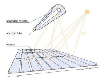
FIGURE 23 Schematic representation of a Linear Fresnel collector [19]
