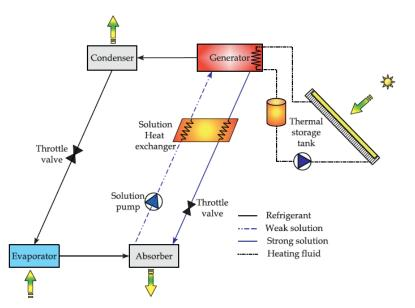
FIGURE 36 A schematic diagram for the basic single effect solar absorption cooling system.[35]
