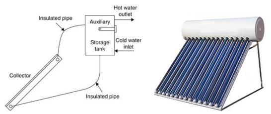
FIGURE 28 Schematic diagram of a thermosiphon FIGURE 29 Thermosiphon system [28] solar water heater [28]
