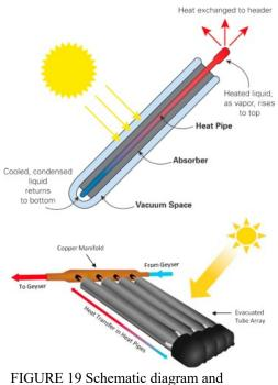
FIGURE 19 Schematic diagram and operating principle of an ETC [19]
