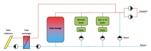
FIGURE 61 Example of combined solar and biomass in parallel configuration[44]
