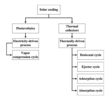
FIGURE 32 Classification of main solar cooling technologies [19].
