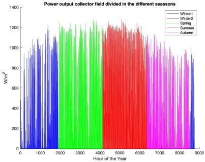
FIGURE 59 Power output collector field by each season
