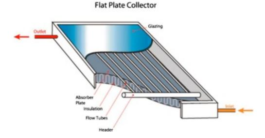
FIGURE 18 Schematic of a typical flat collector [19]
