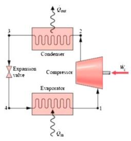
FIGURE 33 Vapor compression system [33].
