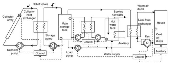
FIGURE 31 Detailed schematic diagram of a solar space-heating and hot water system with antifreeze solution [30].
