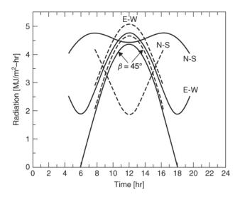
FIGURE 16 Extraterrestrial solar radiation for different tracking modes in both winter(dotted line) and summer(solid line) solstices[14]
