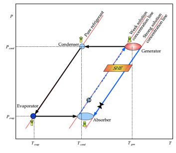
FIGURE 35 A P-T-X diagram of a single effect absorption system. [35]
