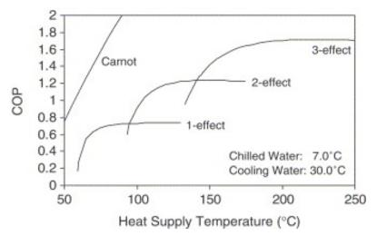
FIGURE 37 Coefficient of Performance (COP) as a function of solar heat supply temperature for single-, double- and triple-effect LiBr–water absorption chillers.[37]
