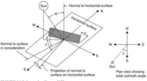
FIGURE 14 Solar angles diagram[13]
