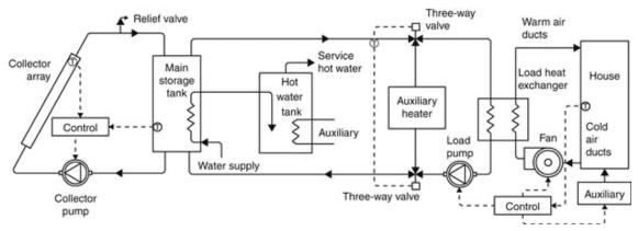
FIGURE 30 Schematic diagram of a solar space-heating and hot water system. [30]
