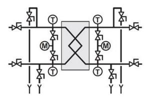
FIGURE 27 Schematic of a heat exchanger [8]
