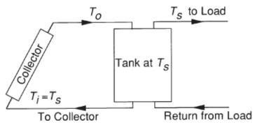
FIGURE 25 A typical system using water tank storage, with water circulation through collector to add energy and through the load to remove energy. [25]
