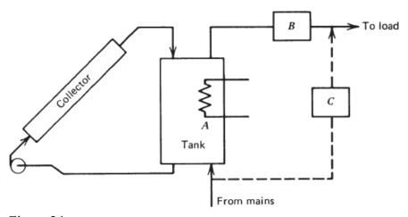
Figure 24 Schematic of alternative location for auxiliary energy supply to a one-tank forced-circulation solar water heater: A, in tank; B, in line to load; C, in a bypass around tank. [24]
