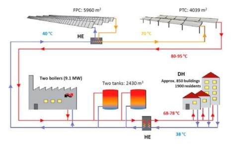
FIGURE 50 Schematic of the operation of the reference solar district heating network [39]
