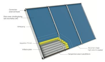
FIGURE 46 Schematic of the solar flat plate collector [40]
