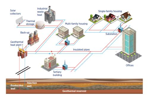
FIGURE 11 Schematic diagram of a district heating system using multiple energy sources [2]
