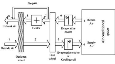
FIGURE 34 Desiccant dehumidification associate with evaporative. [34]
