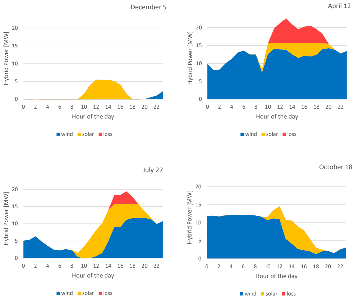
Fig 4.21. Power generation diurnal profile of the hybrid project for selected days
