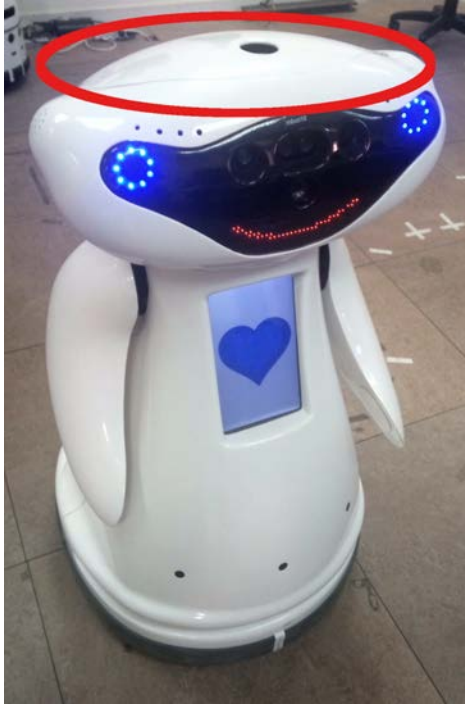
(a) The SO model of the MOnarCH project's robotic platform. The red ellipse marks the zone where the system is installed.
