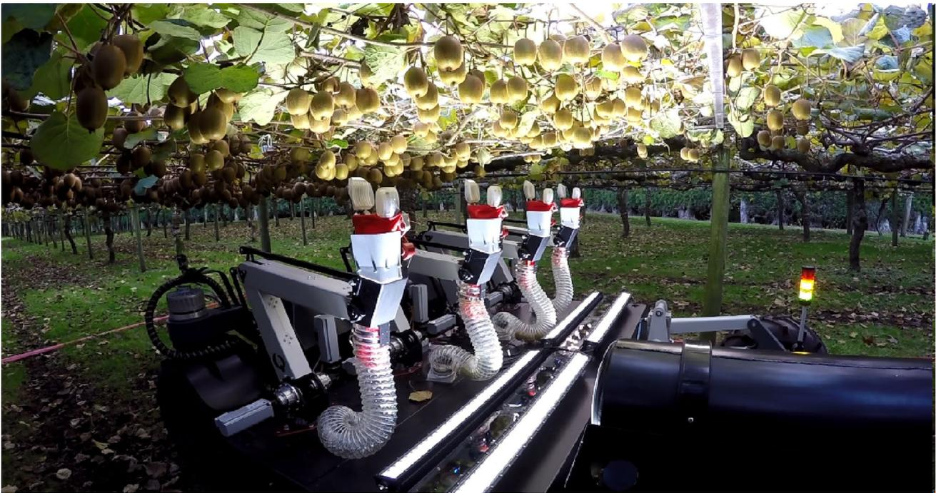
**Fig. 1** The kiwifruit harvesting system with four robot modules
