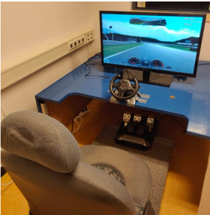
Figure 1 The set-up of the driving simulator used in both the experimental driving and passive viewing control conditions. It consisted of a chair, steering wheel, pedals and a 23-inch flat screen. A PlayStation 3 and the game Gran Turismo (Yamauchi, 2013) were used to simulate the actual driving experience. Participants drove (or viewed a recorded video of) three laps on the Twin Motegi Course.
