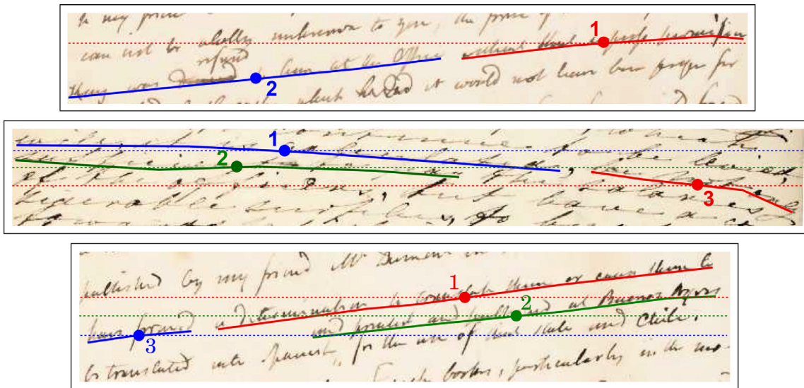
Fig. 7. Real examples from Bentham Papers images 010_003_002, 019_004_003, which illustrate text line splitting errors that affect RO. In the simulation experiments these examples correspond, top to bottom, to Cases 1, 2 and 3.
