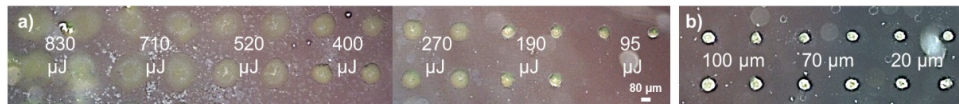
Fig. 2. Images of the photopolymer droplets deposited on the substrate with a picosecond laser: a) at different laser energies and a distance (gap) between donor and substrate of 50 \mu\text{m} ; b) at different distance (gap) between donor and substrate and an energy of 215 \mu\text{J} . All the images were obtained with an optical microscope by using a 5x objective and are sharing the same scale bar.
