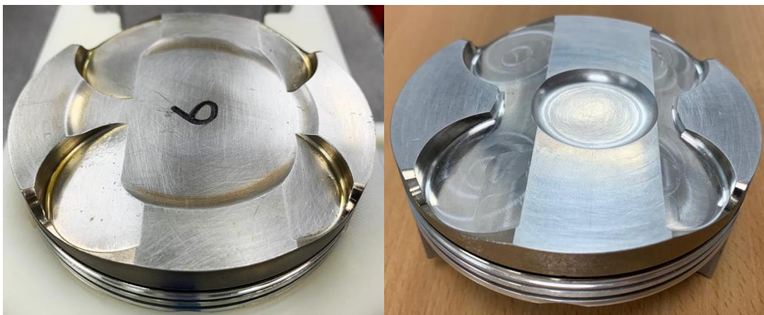
Figure 6-33 Base Piston Crown (L) and Bowl Piston Crown (R) Designs
