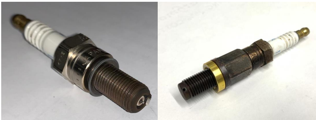
Figure 4-2 M10 Spark Plug Utilised in the Pre-chamber (Left) and Pre-chamber Spark Plug Assembly with Control Washer (Right)
