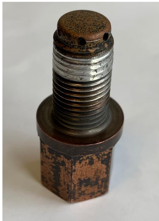
Figure 5-41 Melted Aluminium on the Pre-chamber Thread
