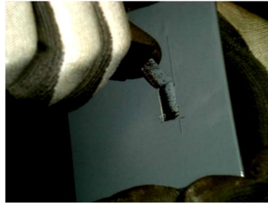
Figure F. 3: grasped raised end due to constant pulling force.
