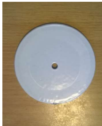
Figure 3. 15: Cylindrical steel plate for abrasion testing.
