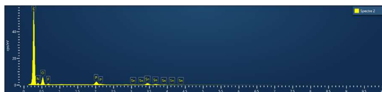
Figure 7. 18: The compositional results of the surface area of spectra 1 (pinhole deep surface) and spectra 2 (defect free surface) by comparative X-ray microanalysis.
