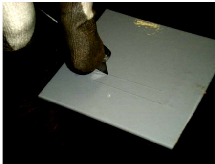
Figure F. 1: Strip delimitation onto the coated plate for adhesion test.
