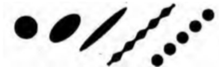
Figure 2. 11: Mechanism of rupture by Rayleigh instabilities [135].
