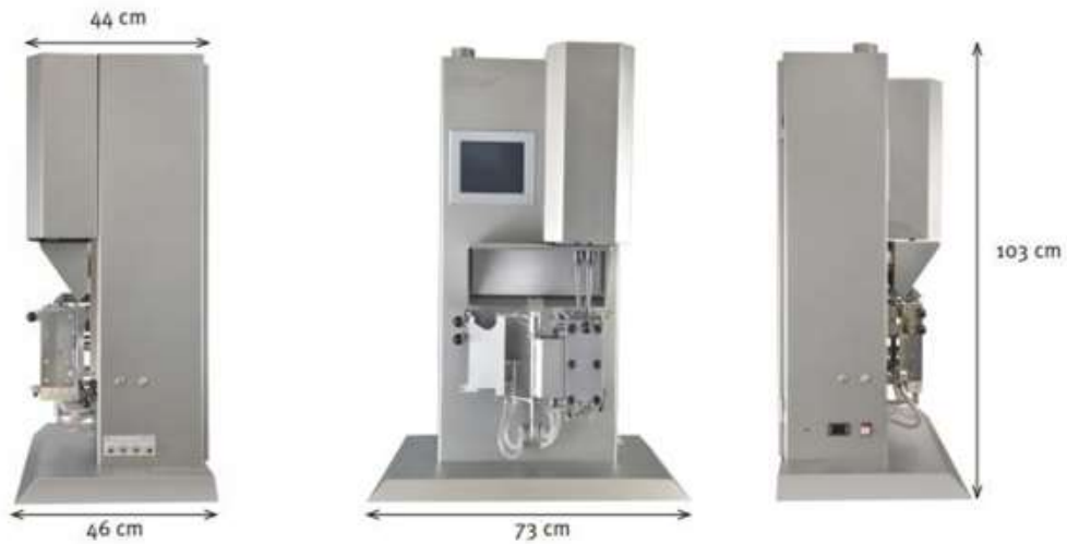
Figure D. 1: Overall dimensions of the twin screw 15 cm 3 Xplore ® Micro-DSM compounder [166].
