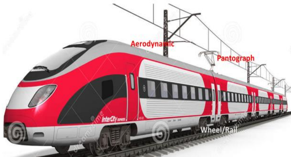
Figure 5.3 Major exterior noise sources on high-speed trains (Source: Adapted from Dewberryjes.blogspot.com., 2019)
