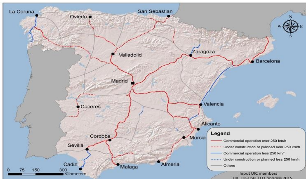
Figure A.5 HSR network in Spain (Source: UIC - International union of railways., 2019d).
