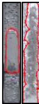
Figure 3.11: Image processing for the extraction of bubble diameter and Taylor bubble length required for volume calculation.
