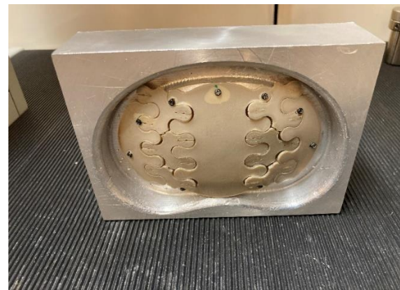
Figure 29. Mechanical testing at the displacement of 6 mm (A). Mechanical testing at the displacement of 8 mm (B). The PEEK prototype of the modular cranial semi-PSI after the test (C) and (D).
