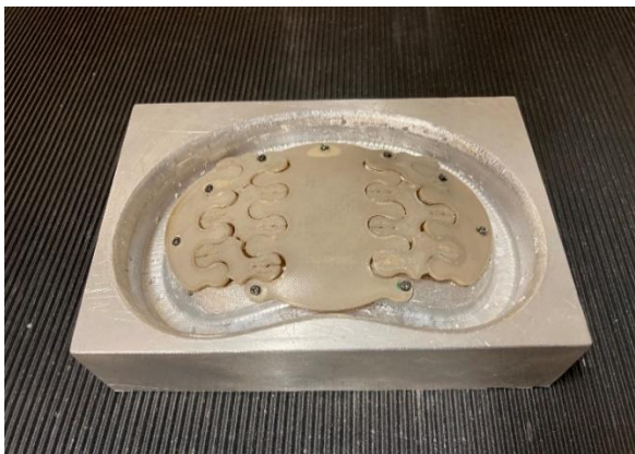
Figure 29. Mechanical testing at the displacement of 6 mm (A). Mechanical testing at the displacement of 8 mm (B). The PEEK prototype of the modular cranial semi-PSI after the test (C) and (D).
