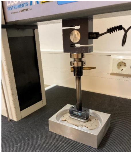
Figure 28. The set-up for the compression test (A). The PEEK prototype of the modular cranial semi-PSI prior to the test.
