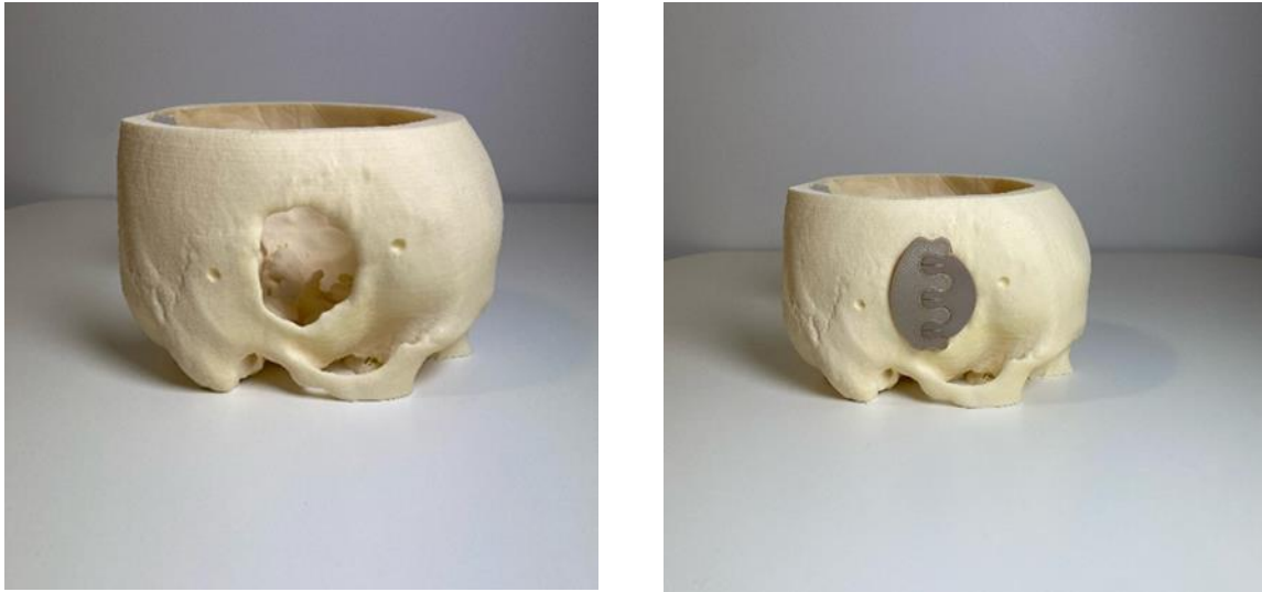
Figure 31. Three modular cranial semi-PSIs are assembled, each tailored to correspond to an anonymized artificial skull produced by AM.
