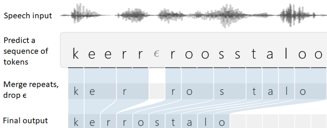
Figure 4: Illustration of CTC decoding [27]. The decoded word was “kerrostalo”. The blank token is \epsilon and was critical in decoding two letters “r”.
