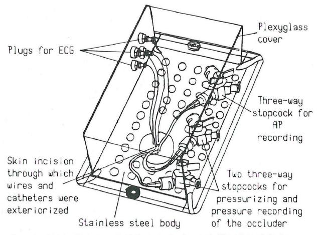
Figure 1. Design and components of the protective box used. Dimensions of the box are  $100 \text{ mm} \times 70 \text{ mm} \times 30 \text{ mm}.$
