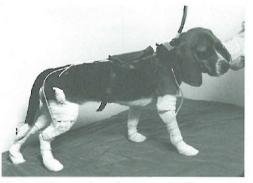
*Figure 2.* The experimental arrangement. The magnetoresistive sensor was attached to the right hindlimb. EMF transducers were attached to the paws by elastic bandage.
