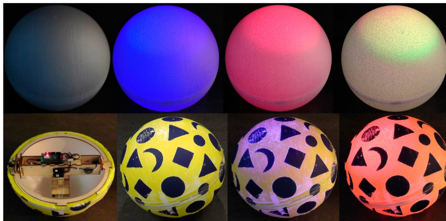
Figure 3. The movable remote controlled interactive ball of 50 cm. The ball is shown emitting different colours, both with the painted (blue yellow / high contrast) and a more transparent white outer shell.
