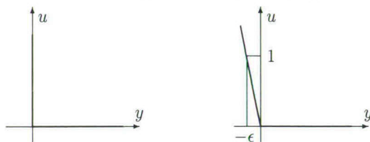
Figure 5.1: Complementarity characteristic and one of its possible approximations
