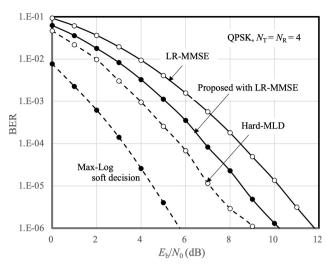
Fig. 7 MMSE based soft decoding compared with MLD based ones.
