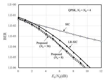
Fig. 2 BER performance of proposed soft decoding with SIC.
