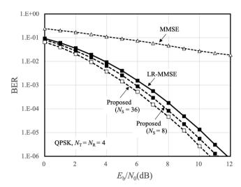
Fig. 1 BER performance of proposed soft decoding with MMSE.
