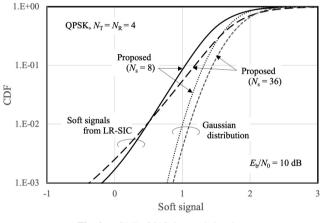
Fig. 4 CDF of SIC detected signals.
