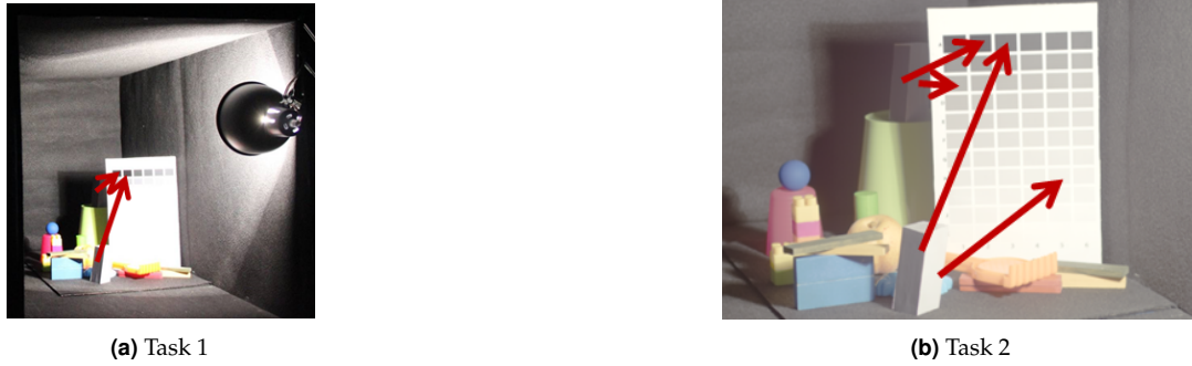
Fig. 2. In Experiment 1, observers performed two tasks. In Task 1 (Figure 2a), observers had to match the brightnesses of the 5 cuboids' facets to the brightnesses of 5 patches in the reference table. In Task 2 (Figure 2b), observers had to perform the same task on the TMO image displayed on the calibrated monitor. (Red arrows are randomly drawn just for illustrative purposes).
