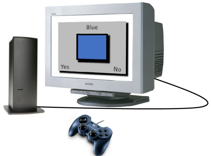
Fig. 13 Setup for our psychophysical experiment. Color patches and color names were presented on a calibrated CRT monitor and the observer pressed buttons on a gamepad to decide whether the color patch was well described by the name or not. The background was mid-grey and a reference white was provided by a D65-colored frame
