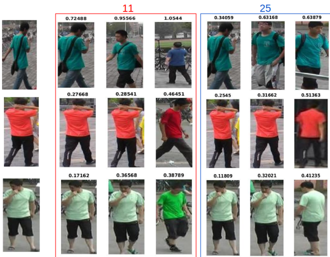
Fig. 12 Examples for top 3 ranking with 11 and 25 color terms. Note that some of the errors which occur when using 11 color names are resolved when using 25 color names.
