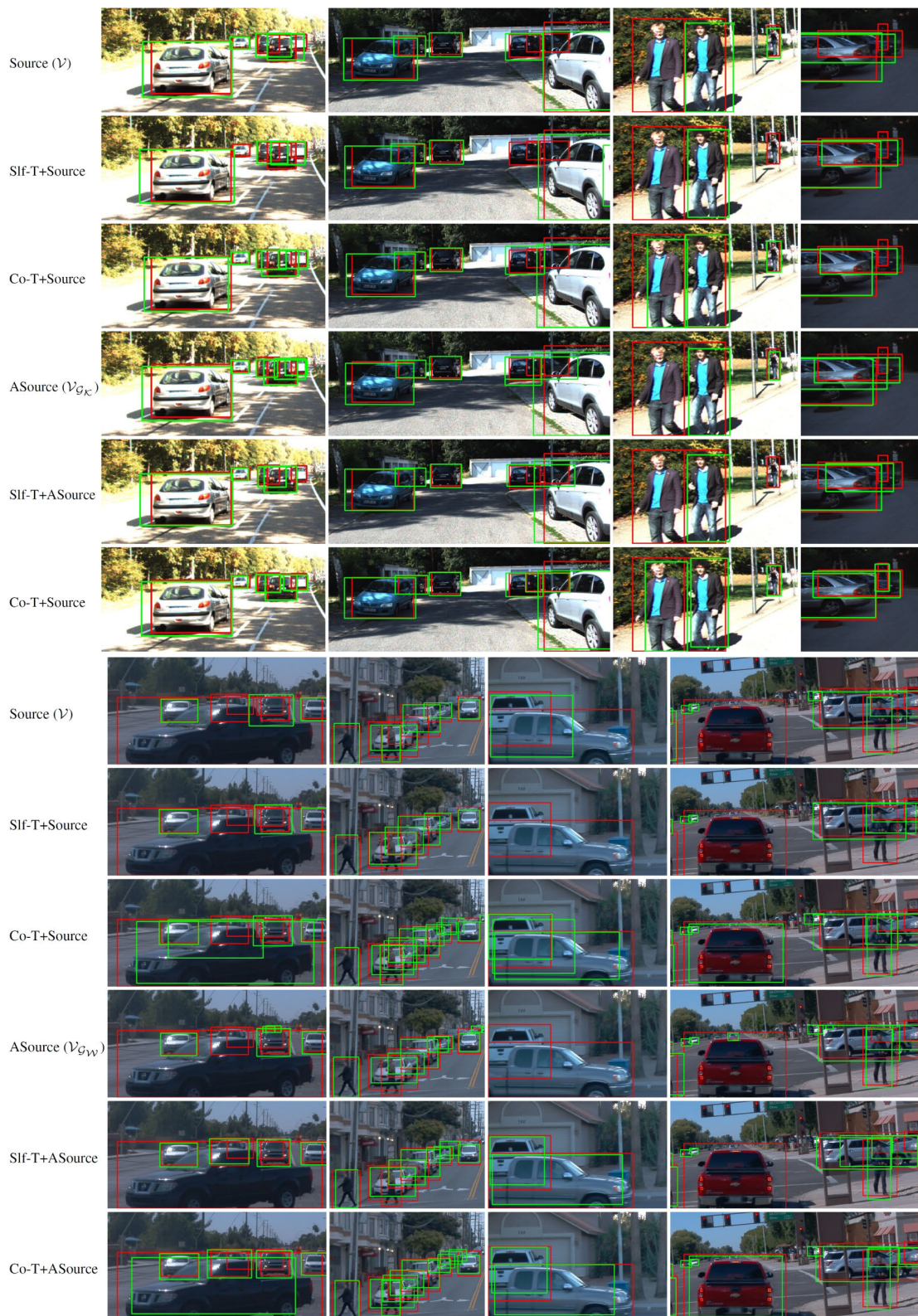
FIGURE 11. Results for \mathcal{K}^{tt} (top ‘Source \rightarrow Co-T + ASource’ block) and \mathcal{W}^{tt} (bottom ‘Source \rightarrow Co-T + ASource’ block). Red BBs are the ground truth, and green ones are the detections done by the detector indicated at the first column of each row.
