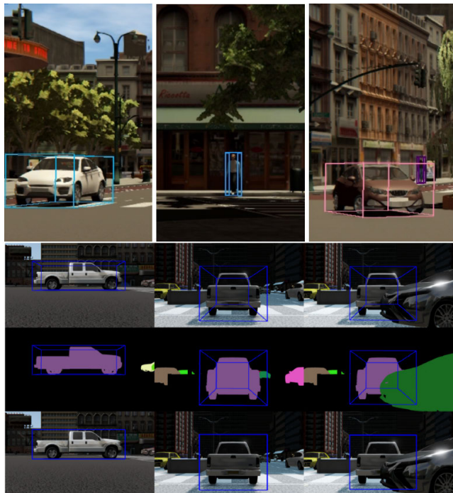
FIGURE 3. Top images: virtual-world patches showing 3D BBs framing vehicles and pedestrians. Bottom image: projecting 3D BBs as 2D BBs for different views of a pickup, with instance segmentation as visual reference.
