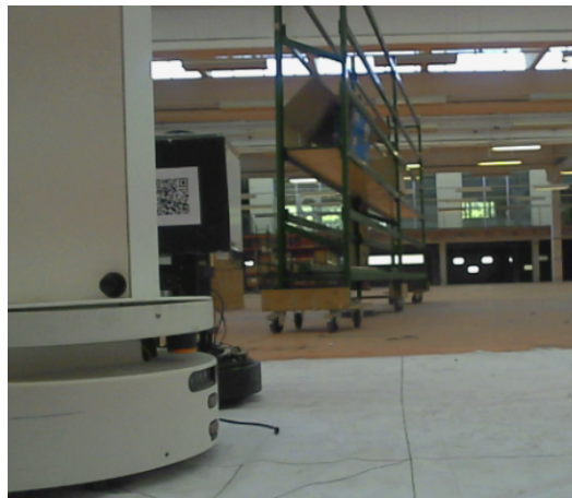
(b) Fail detection of the Pawn using the QR-code pose estimation method.
