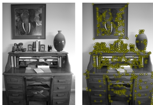
(b) Example of “Harris Corner Features” detected in an image.
