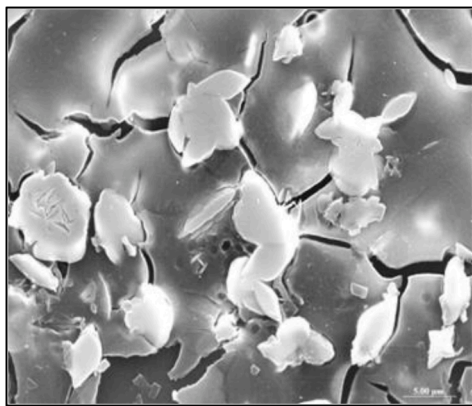
Fig. 4. Microstructure (after chemical etching of polished surfaces with HF solution) of the monomineral glass-ceramics in Di: CaTs series, heat treated 850 °C: augite crystals embedded in the glassy matrix.
