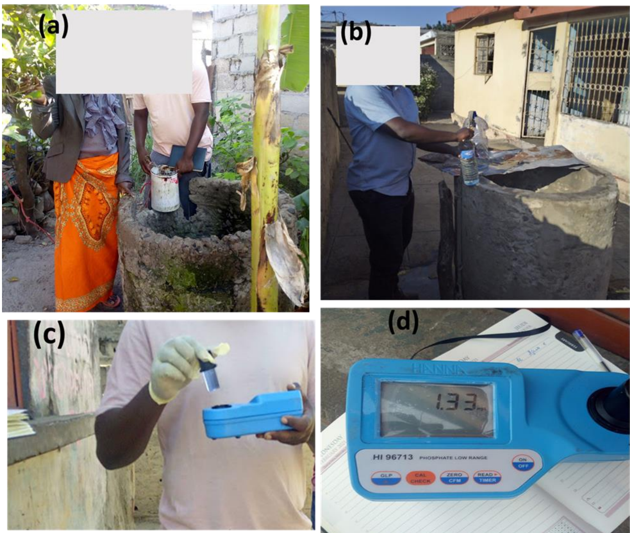
Figure S1. Sampling and chemical analysis of well water S1. (a) Water collection - South well (b) Water collection - North well; (c) Chemical analysis process (d) Result of phosphate analysis.
