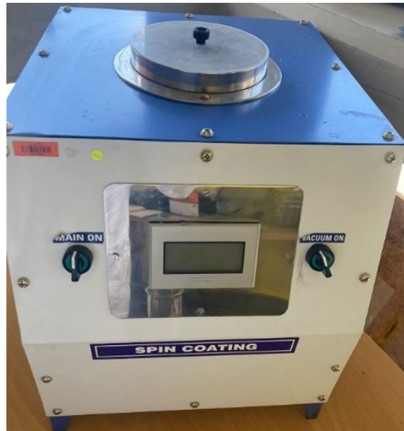
Figure 2.3: The photograph of a spin coating machine available at UNISA
