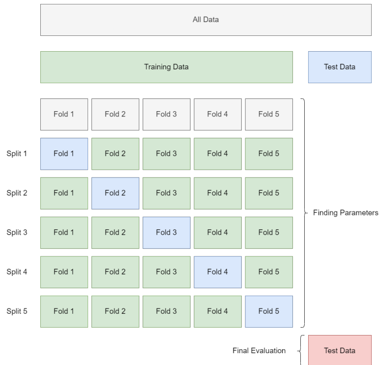
Figure 4.3: A K fold example. This approach will split the data provided into k groups, defined by the user, afterwards it will select one group as a test set and the remaining groups are used as training sets, and repeats this process until every group has been used as a test set in evaluation.
