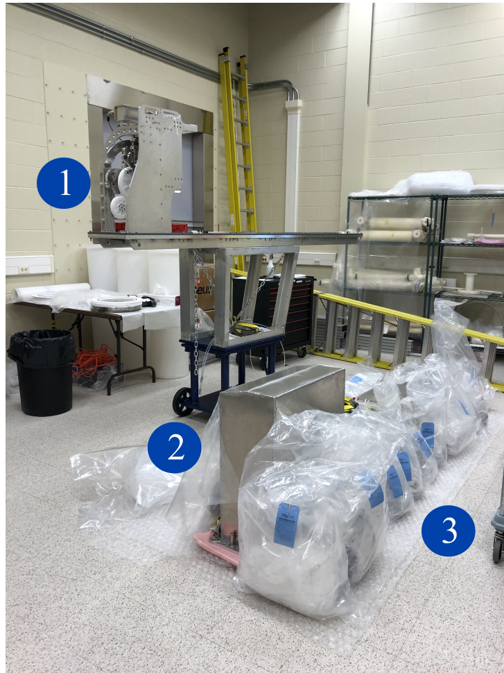
Figure 3.15: Disassembled URM in the SNOLAB surface clean room: 1) URM base plate and drive systems, 2) cover, 3) internal parts stored in triple heat-sealed bags for transport.
