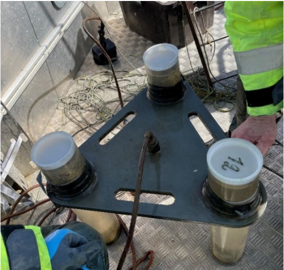
Figure 9. A collector of sinking matter and a collection tube at the end of the sampling period.
