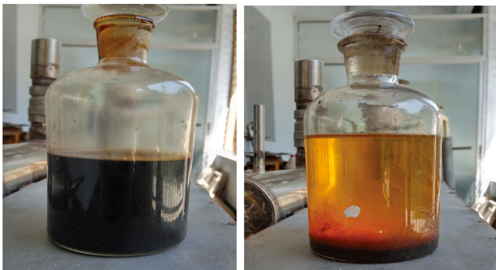
Fig. 2. (a) Crude waste tyre pyrolysis oil (b) Distilled waste tyre pyrolysis oil.
