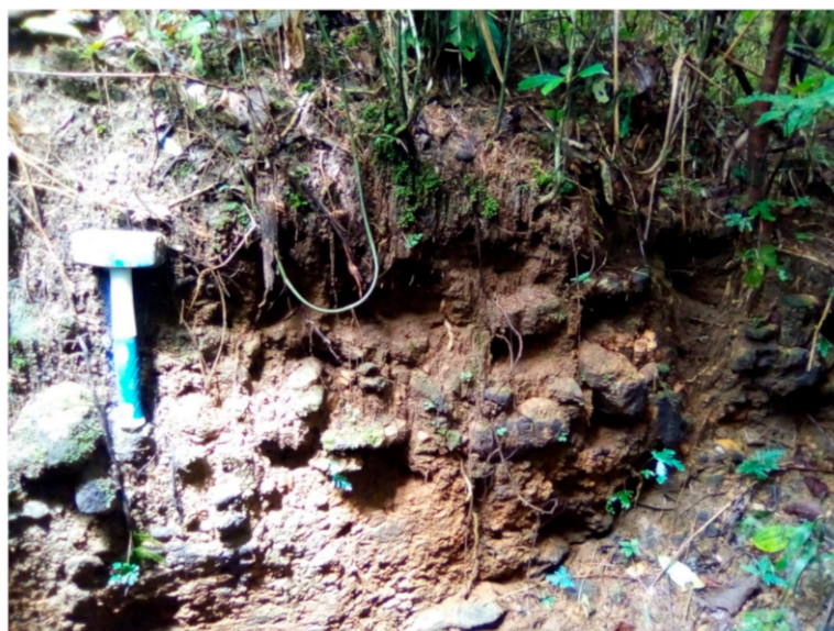
Figure 17. Section of a 2-m excavation dug parallel to the E–W direction for sampling resistant boulders rich in Mn at Neghe village (Hammer used as the scale is 25 cm long).
