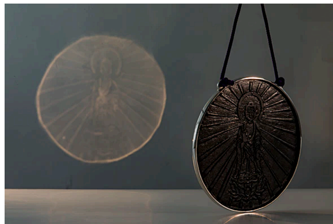
Fig. 4. Photo of the visual image and the projected Makyoh image of a modern Japanese mirror replica (with kind permission from kyotocrafts.store, © 2020, Kyoto Crafts Store).
