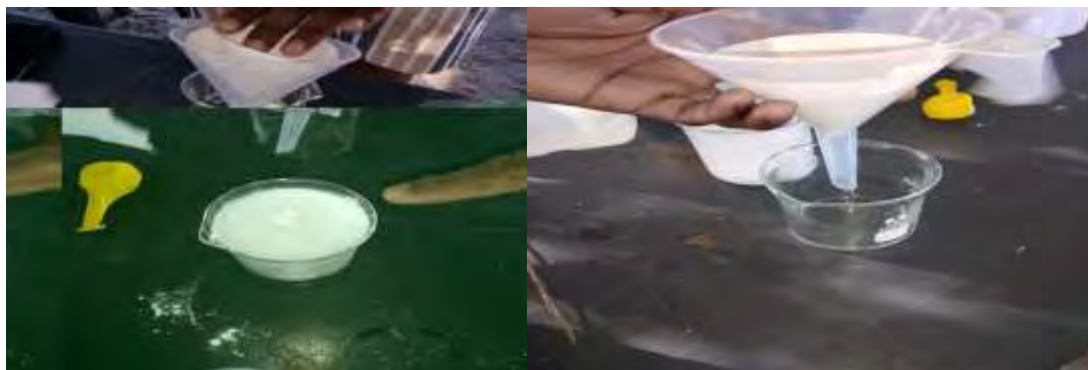
Figure 7.14: Shows the process of making lime water and filtration to obtain a clear solution
