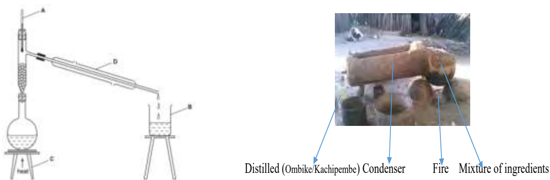
Figure 6.1: Conventional fractional distillation apparatus and traditional fractional distillation apparatus
