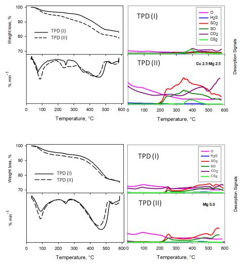
Figure 2. 13 Comparison of weight loss % and species release during TPD tests under Ar flux from H<sub>2</sub>S saturated modified AC after few minutes (TPD (I)) and two months (TPD(II)) respectively later H<sub>2</sub>S adsorption tests. Derivative curves (down) of weight losses.
