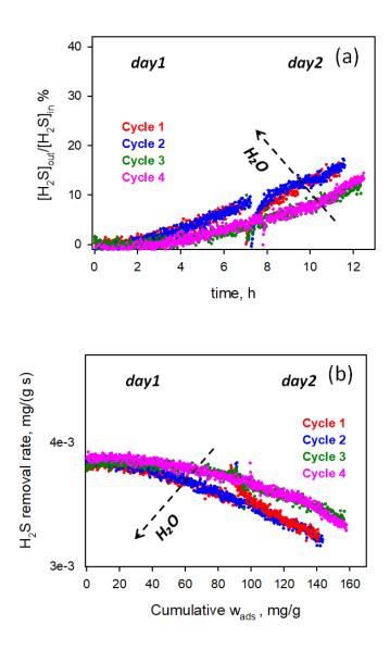
Figure 2. 19 Breakthrough curves (a) and apparent  $H_2S$  removal rate (b) of Cu2.5Mg2.5-modified monolith for  $H_2S$  after four cycles of adsorption tests at T=30°C, P=1 atm in presence of humidity (HR=50%) and O<sub>2</sub>=2500 ppm and subsequent TPD at T=600°C in N<sub>2</sub>
