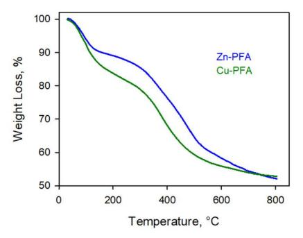
Figure 3. 6 Weight loss as a function of temperature of Zn- and Cu-activated PFA under N2 flow
