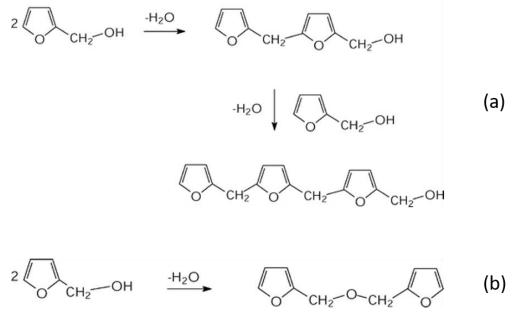
Figure 3. 2 Condensation Reaction Schemes between the OH of the Methylol Group of One Furan Ring and (a) the 5-Position of Another Furan Ring and (b) the Methylol Group of Another Furan Ring (Bertarione et al., 2008)
