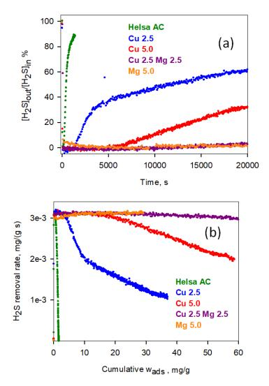
Figure 2. 10 Comparison of breakthrough curves (a) and apparent H<sub>2</sub>S removal rate (b) of monoliths for H<sub>2</sub>S capture at T=30°C, P=1atm in presence of humidity (HR=50%) and O<sub>2</sub>=2500 ppm
