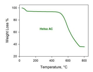
Figure 2. 3 Weight loss as a function of temperature of Helsa AC monolith under air flow
