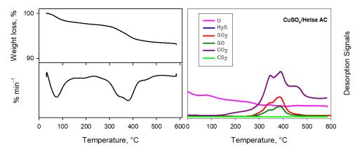
Figure 2. 14 Weight loss % and species release during sulphates decomposizion under N<sub>2</sub> flux from CuSO<sub>4</sub> impregnated on AC
