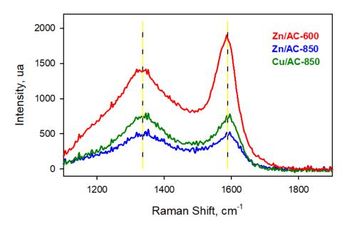
Figure 3. 10 Raman spectra of Zn/AC-850, Zn/AC-600 and Cu/AC-850
