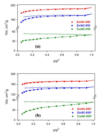
**Figure 3. 11**  $N_2$  physisorption isotherms at 77 K for activated carbons pyrolyzed under pure helium (a) and under  $O_2$ /He mixture (b) (closed symbols for adsorption branch, open symbols for desorption branch)
