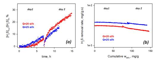
**Figure 2. 12** Effect of inlet flow rate on breakthrough curves and the apparent  $H_2S$  removal rate of Cu2.5Mg2.5 by varying inlet flow rate at P=1 atm in presence of humidity (HR=50%) and  $O_2$ =2500 ppm
