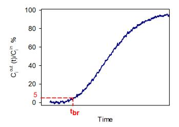
Figure 1. 3 Breakthrough curve in a fixed bed reactor
