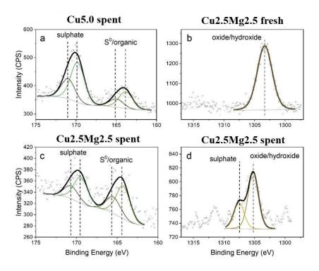
Figure 2. 18 XPS spectra in S2p spectral region of spent Cu5.0 and Cu2.5Mg2.5 sorbents (a and c) and in the Mg1s region of fresh and spent Cu2.5Mg2.5 (c and d).
