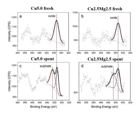
Figure 2. 16 XPS spectra in Cu2/p spectral region of fresh (a and b) and spent (c and d) Cu5.0 and Cu2.5Mg2.5 sorbents.
