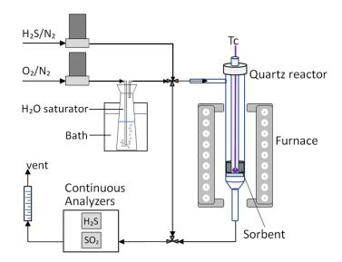
Figure 2. 2 Schematic representation of the experimental equipment used for H<sub>2</sub>S adsorption tests
