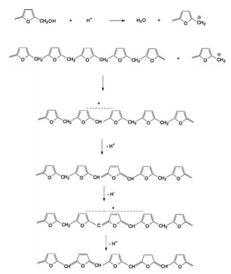
Figure 3. 3 Scheme of reactions responsible of progressive darker colour of the solutions in which acid-catalyzed polycondensation of the FA occurs (Bertarione et al. 2008)
