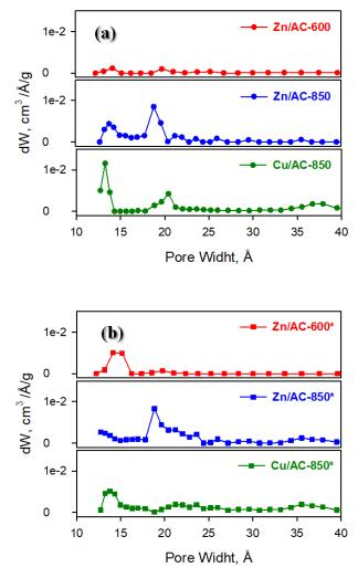
Figure 3. 12. The effect of the composition of the pyrolysis gas on the PSD in the micro/mesopores region
