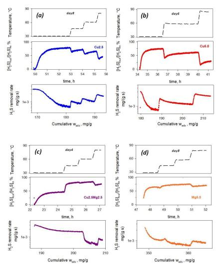
$\label{eq:Figure 2.11} \begin{tabular}{ll} Figure 2.11 \\ Effect of temperature on the $H_2S$ adsorption capacity $nd$ the apparent $H_2S$ removal rate of $Cu2.5$ (a), $Cu5.0$ (b), $Cu2.5Mg2.5$ (c) and $Mg5.0$ (d) $\end{tabular}$
