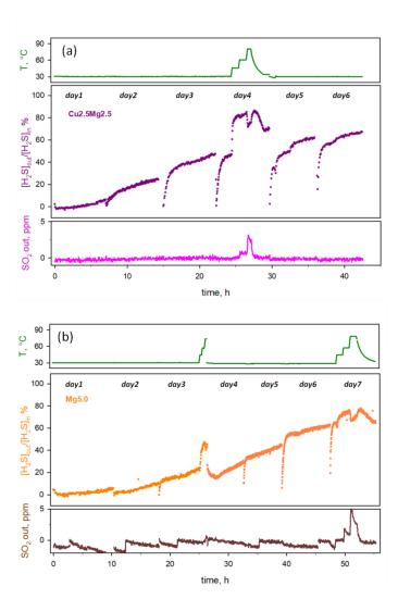
Figure 2. 8 Breakthrough curves of 2.5% wt (a) and 5% wt (b) Mg-modified monoliths for H<sub>2</sub>S capture and SO<sub>2</sub> formation during adsorption test by varying T at P=1 atm in presence of humidity (HR=50%) and  $O_2$ =2500 ppm
