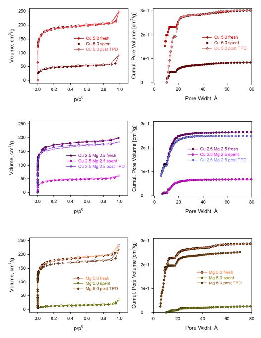
Figure 2. 15 N<sub>2</sub> physisorption isotherms at 77K and PSD for fresh and spent modified monoliths
