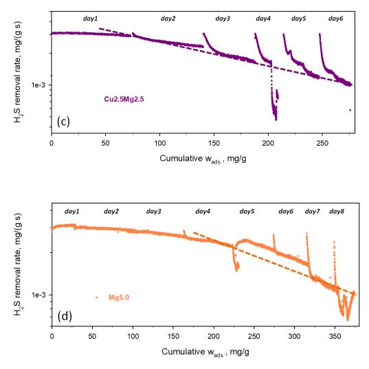
**Figure 2. 9** Trend of apparent H<sub>2</sub>S removal rate over time of Cu2.5 (a), Cu5.0 (b), Cu2.5Mg2.5 (c) and Mg5.0 (d) (solid line). A master line (dashed line) connecting the values of H<sub>2</sub>S removal rate at the end of each day is reported.
