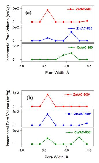
Figure 3. 14. The effect of the composition of the pyrolysis gas on the PSD in the ultra-micropore region
