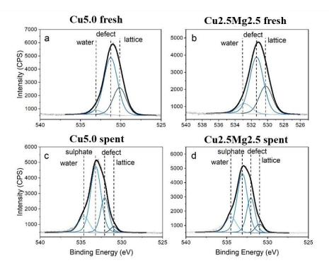
Figure 2. 17 XPS spectra in O1s spectral region of fresh (a and b) and spent (c and d) Cu5.0 and Cu2.5Mg2.5 sorbents
