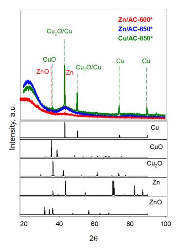
**Figure 3. 9** XRD patterns of Zn/AC-850\*Zn/AC-600\*and Cu/AC-850\*. In the lower graph patterns of reference Zn (PDF 1-1244), ZnO (PDF 36-1451, Cu (PDF 4-836), Cu<sub>2</sub>O (PDF 5-667) and CuO (PDF 45-937) are reported
