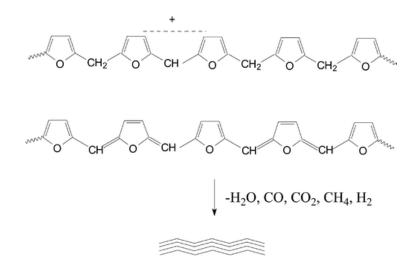
Amorphous carbon Figure 3. 4 Scheme of amorphous carbon formation (Bertarione et al. 2008)
