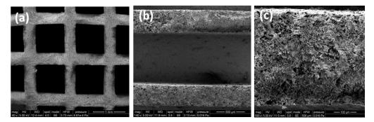
Figure 2. 4 SEM images of monolith cross section (a) at increasing magnifications (channel with two adjacent walls (b); wall (c))
