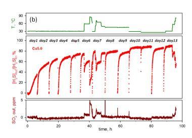
Figure 2. 7 Breakthrough curves of 2.5% wt (a) and 5% wt (b) Cu-modified monoliths for  $H_2S$  capture and  $SO_2$  formation during adsorption test by varying T at P=1 atm in presence of humidity (HR=50%) and  $O_2$ =2500 ppm
