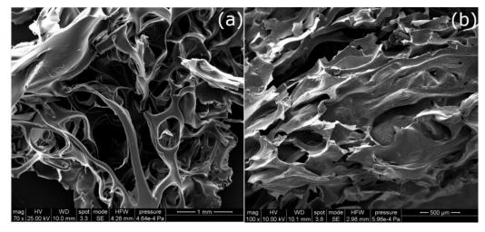
Figure 3. 7 SEM images of Zn/AC-850 (a) and Cu/AC-850 (b)
