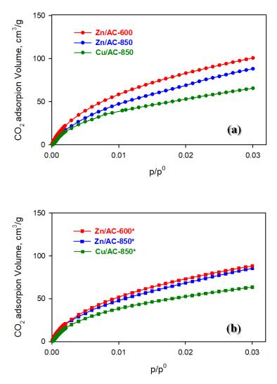
Figure 3. 13 CO<sub>2</sub> physisorption isotherms at 273 K for activated carbons pyrolyzed under pure helium (a) and under O<sub>2</sub>/He mixture (b)
