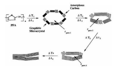
Figure 3. 1 Evolution of the carbon structure deriving from the polymerization of FA (Wang and Yao, 2006)
