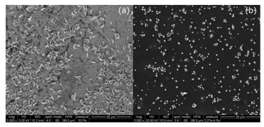
Figure 3. 9 SEM images of Zn/AC-600 (a) and Cu/AC-600 (b) with a greater magnification
