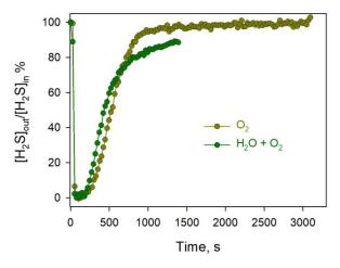
Figure 2. 6 Breakthrough curves of AC monolith in dry and wet conditions. Inlet conditions:  $[H_2S]$ =100ppm,  $[O_2]$ =2500ppm, T=30°C, P=1 atm
