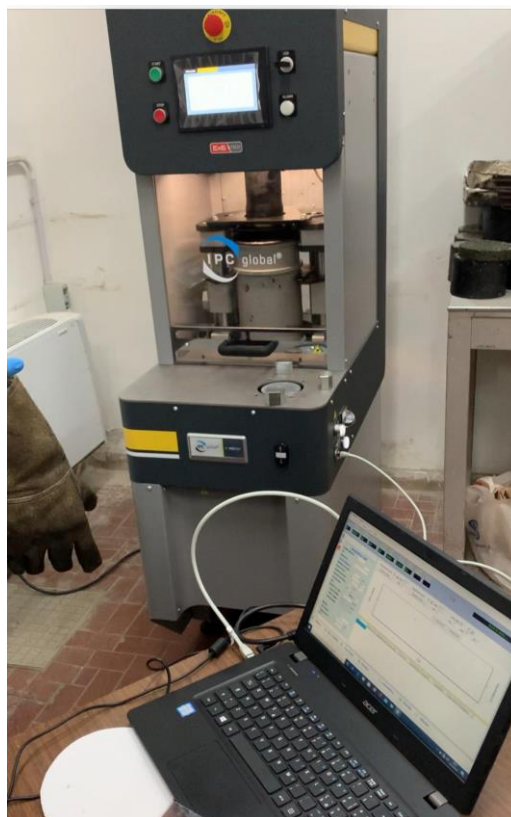
Figure 7.35 Gyratory compactor available at La.Stra
