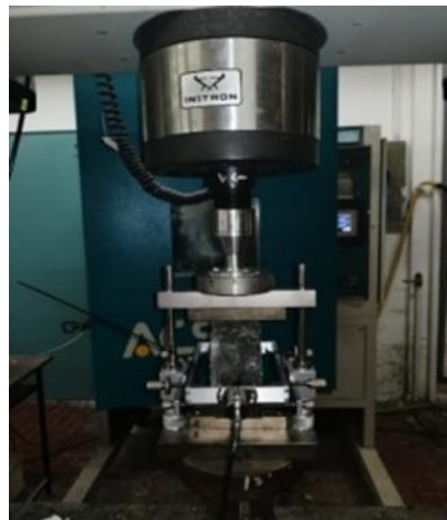
Figure 7.40 ITSM device available at La.Stra
