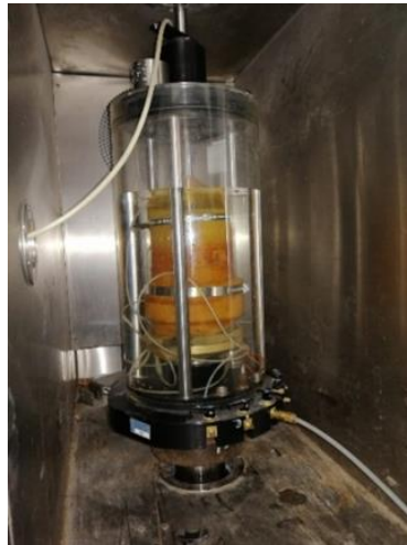
Figure 7.43 Triaxial Cyclic compression device available at La.Stra.
