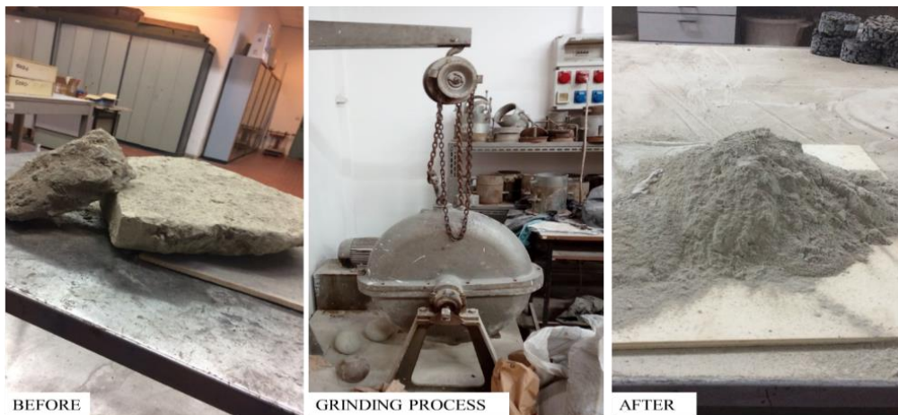
Figure 7.2 Jet grouting waste before and after grinding process
