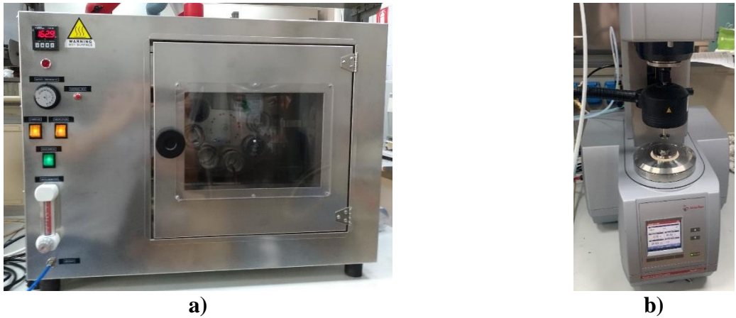
Figure 7.8 La.Stra device: a) RTFOT and b) DSR
