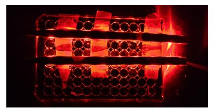
**Figure 4.4.** Experimental setup for NADH photooxidation. Solutions were placed only in the wells under LEDs diode: in the specific experiment line B and D; wells no. 1,3,5,7,10 e 12.
