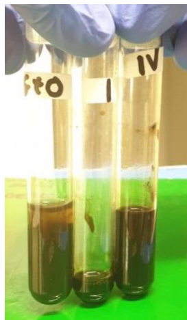
Figure 42: water-based slurry of GtO (8 mg/mL) and of the supernatant (I) and subnatant (IV) part of GO, i.e. the first sample after ultrasonication and centrifugation.
