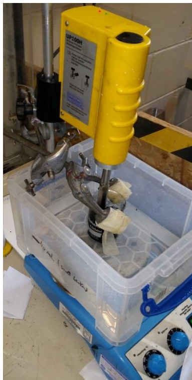
Figure 33: Exfoliation of GtO in water-based slurry with a probe sonicator, with freezing water to prevent excessive heating and the help of a magnetic stirrer.
