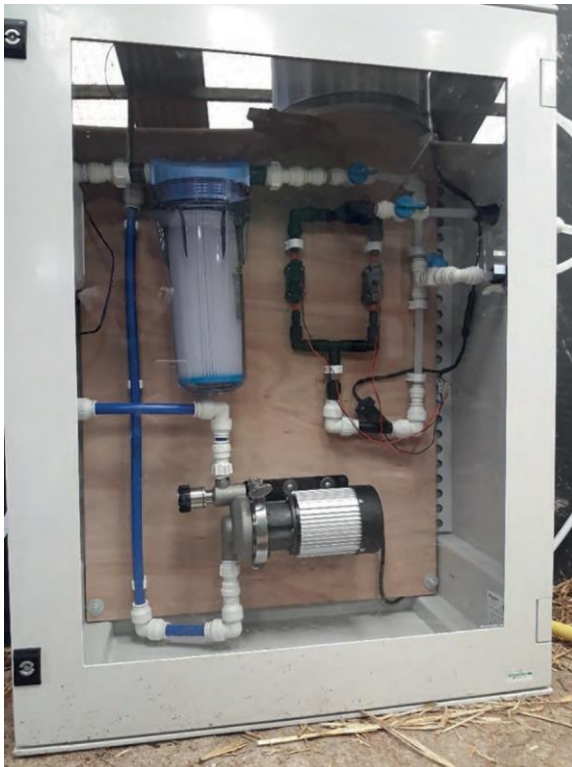
Figure 5.5 Ozone farm box system installed in the Aberdeen Angus farm (Salisbury, UK).
