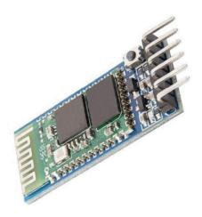
Figure 64 Bluetooth module used HC-05
