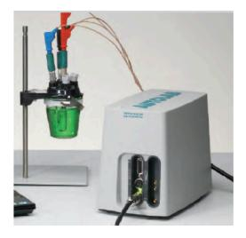
Figure 27. AUTOLAB PGSTAT302N (potentiostat/galvanostat) by Metrohm
