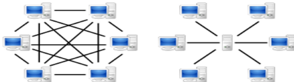
Fig. 2 Shows decentralized forwarding architecture described in P2P network (Fire Chat) vs centralized architecture described in Client/Server network
