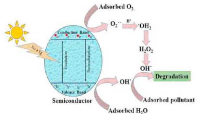
Fig. 18. Mechanism of the semiconductor-based photocatalytic process [291].
