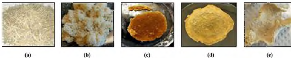
Fig. 1. Physical images of the samples used and modified, (a) untreated sugarcane bagasse, (b) extracted cellulose, (c) regenerated cellulose (RC), (d) cellulose-glutaraldehyde (C-GA) and (e) cellulose-glutaraldehyde-poly(vinyl alcohol) (C-GA-PVA) hydrogels.
