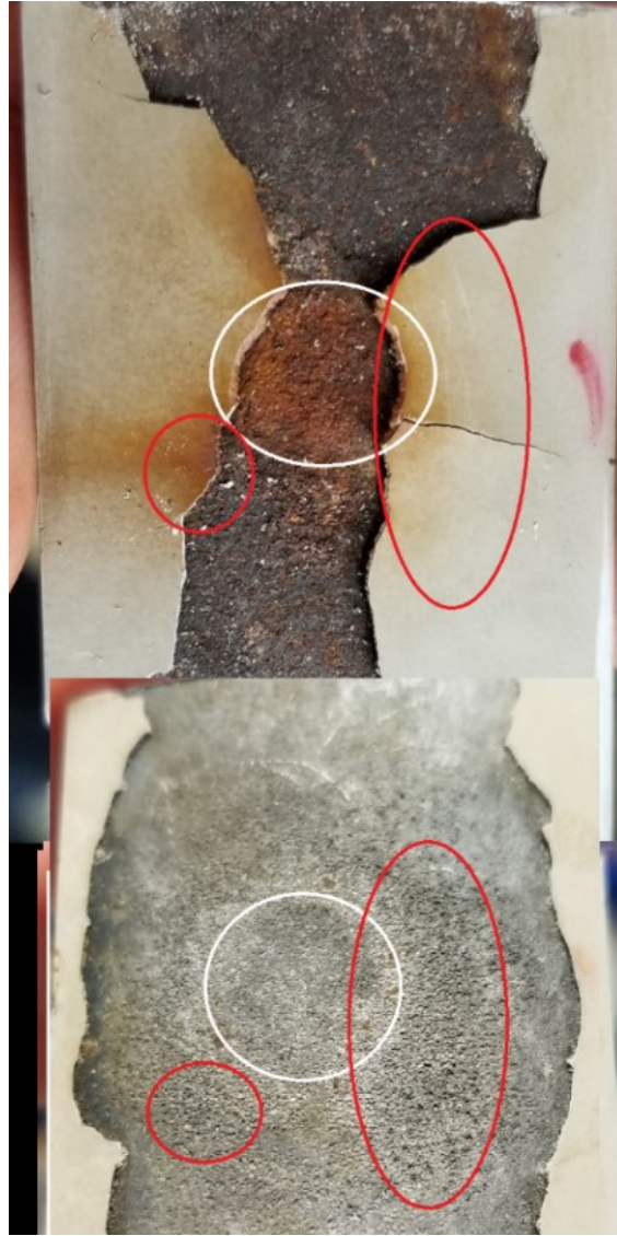
Figure 3.11: Pipe 20 which had one paint section damaged. Red circles were deepest pits. They occurred here perhaps due to the lack of free flow O_2 , while away from the open surface, and away from the area still protected by coating but no electrolyte ingress.
