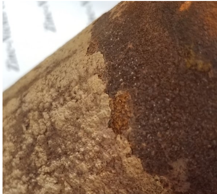
Figure 4.8: Early exfoliation, typical outer (lightly bound) and inner (strongly bound) oxides.
